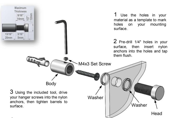
4 Screw threaded studs into your barrels, then place your panel in position and thread on caps until snug.
