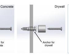
Always check the installation surface to ensure that the substrate will be strong enough to hold the weight of the panel. All installation must be done so with proper hardware and protective gears to ensure safety. It is important to check that parts are properly tightened at the end of each installation.
