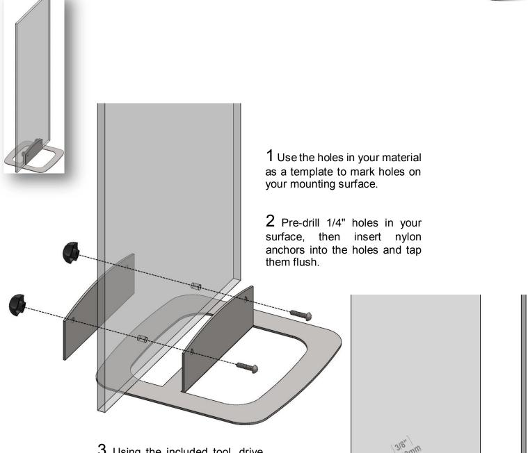
3 Using the included tool, drive your hanger screws into the nylon anchors, then tighten barrels to surface.
