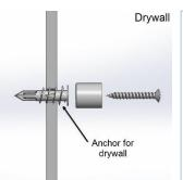
Always check the installation surface to ensure that the substrate will be strong enough to hold the weight of the panel. All installation must be done so with proper hardware and protective gears to ensure safety. It is important to check that parts are properly tightened at the end of each installation.
