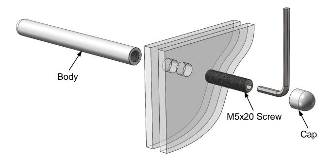
4 Screw threaded studs into your barrels, then place your panel in position and thread on caps until snug.
