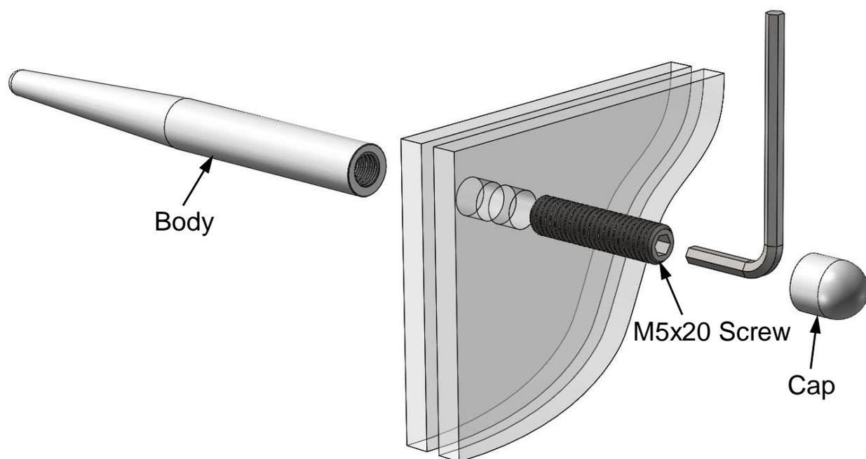
**4** Screw threaded studs into your barrels, then place your panel in position and thread on caps until snug.
