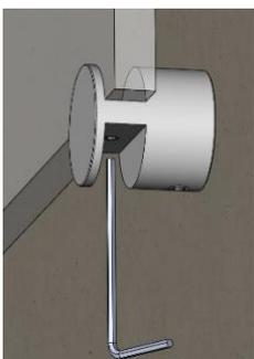
**4** Slide the panel all the way through the edge grips and tighten the M4 set screw on the inside edge of the edge grip to secure the panel to the edge grip. Ensure it is a snug fit but it does need to be overtightened.
