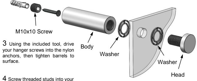
4 Screw threaded studs into your barrels, then place your panel in position and thread on caps until snug.
