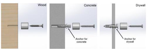
Always check the installation surface to ensure that the substrate will be strong enough to hold the weight of the panel. All installation must be done so with proper hardware and protective gears to ensure safety. It is important to check that parts are properly tightened at the end of each installation.
