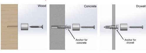
Always check the installation surface to ensure that the substrate will be strong enough to hold the weight of the panel. All installation must be done so with proper hardware and protective gears to ensure safety. It is important to check that parts are properly tightened at the end of each installation.
