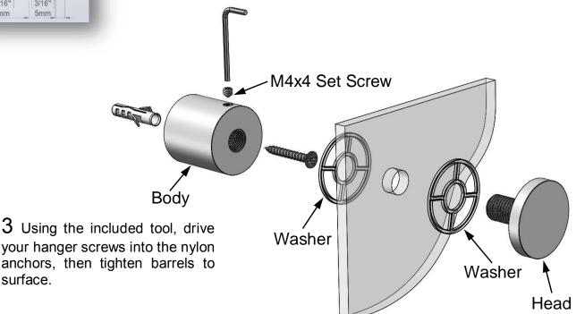
4 Screw threaded studs into your barrels, then place your panel in position and thread on caps until snug.
