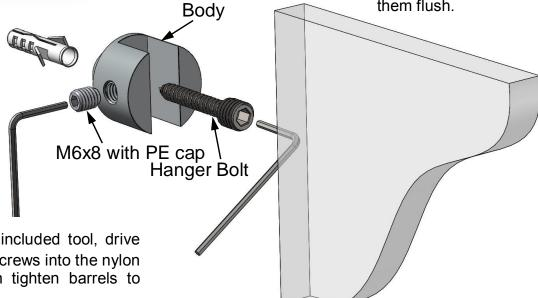
3 Using the included tool, drive your hanger screws into the nylon anchors, then tighten barrels to surface.
