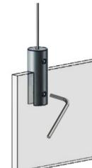
4 With the fork(s) attached to the cable you can attach your panel to the forks. Unscrew the set screw, position your panel in place and secure the set screw. *Note: The stainless steel forks will have washers to protect your panel.*
