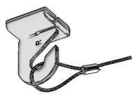
2 Take the looped end of your cable and put it over the TCLAMP hook. Take your cable and cut the cable to the desired length. Allow extra to be screwed into the hanging forks.
