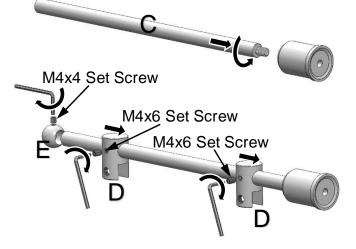
**5** To apply your sign remove the M6 set screws from the panel grips (Part D). Slide the Sign in pace and tighten down the M6 set screws firmly.
