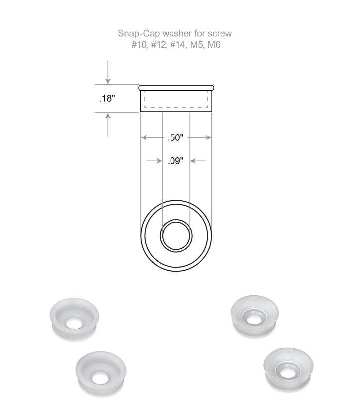
Washer for flat head Washer for countersunk screw use Item #: W10/12FB screw use Item #: W10/12CS
